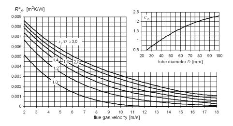
Estimating fouling factors introduces a considerable uncertainty into exchanger design; the value assumed for the fouling factor can overwhelm the accuracy of the predicted values of the other coefficients. Fouling factors are often wrongly used as factors of safety in exchanger design.
